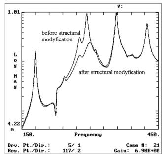
Figure 7. Comparison of the frequency response function before and after introduction of the structural modification
