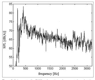
Figure 8. Noise spectra (in dB [A]) at the grain crusher operator's workstation during grain crushing for initial condition
