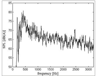
Figure 9. Noise spectra (in dB [A]) at the grain crusher operator's workstation during grain crushing after increase in stiffness coefficients
