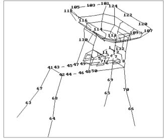
Figure 6. Geometric model of grain crusher introduced to the experimental modal analysis system
