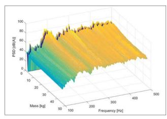
Figure 2. Sound pressure level (SPL) dB(A) spectra at work station of a grain crusher operator as a function of filling the hopper with wheat grain
