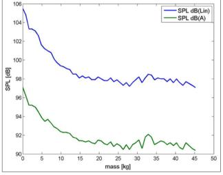
Figure 1. Comparison of sound pressure level (SPL), dB(linear) and A-weighted dB(A) at the work station of a grain crusher operator
