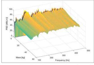
Figure 3. Sound pressure level (SPL) dB(Lin) spectra at work station of a grain crusher operator as a function of filling the hopper with wheat grain
